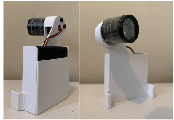
Fig. 2. Proposed QLF prototype
